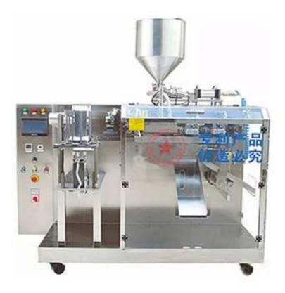
This tomato kechup premade pouch packing machine (hot sauce spout pouch filling sealing machine) is a low cost mini pick fill seal machine. It does spout pouches, premade bags filling and packaging automatically.
