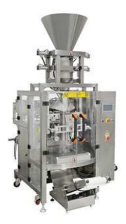
Automatic completion of measuring, bag making, filling, sealing, cutting and printing codes. Pack different grains or granules, such as sugar, salt, desiccant, coffee, washing powder, glucose, seeds, seasoning, pepper, beans, etc.
