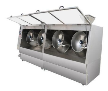
This machine is widely applied to the tablet, ball and pill materials polishing process in the industry of pharmaceutical, food and chemical.
