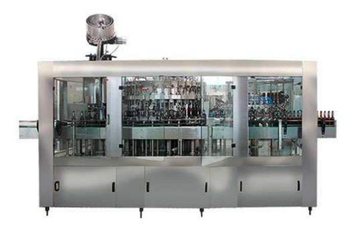
HEM design 40-40-10 beer bottle rinsing filling capping machine adopts Counter pressure filling technology, this machine is specially designed for beer filling. The machine has the advantages of high speed, reliable output, compact design and stable operation. The machine is suitable for medium or large capacity breweries.
