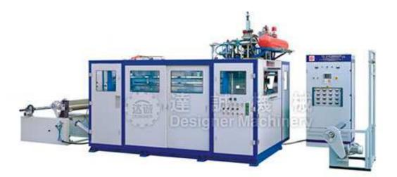
We are a professional plastic sheet thermoforming machine (standard type) supplier in China. This kind of machine is mainly used to make PP, PS, PET and PE package containers for food.
