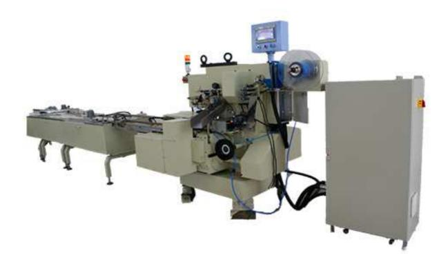
Top Twist Packing Machine are applied in the full automatic packaging of chocolate, pralines and pressed candies. With the twist joint on the top, it can be used for packing the product with a special size and shape. Package speed can be up to 260 grains per min at most, which depends on the product shapes and package material
