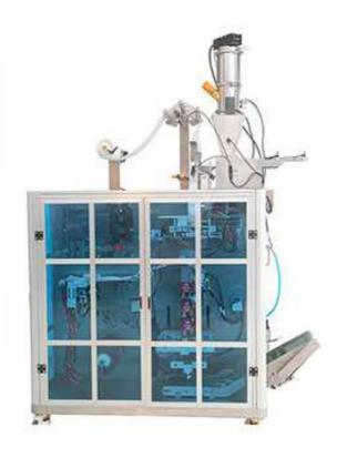
The standard commercial coffee packing machine, Adopts the 3-side ultrasonic sealing for tea bags, Besides, equips with the SCREW feeder & weigher, with the advantage of HIGH ACCURACY(Reaches  $\pm$  0.2 grams/bag), also for easier operation.
