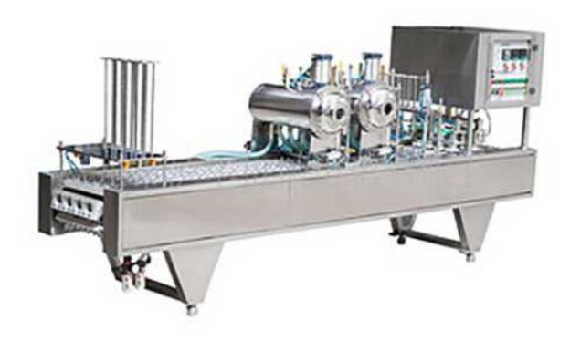
The machine is suitable for all kinds of plastic cup, bowl, plastic composite film or aluminum plastic composite film for heat sealing and cutting edge. Such as jelly, milk, tofu etc.
