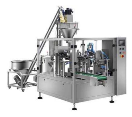
This equipment mainly consists of prefabricated bags fully automatic rotary packing machine, auger filler and auger conveyor. Suitable for milk powder, coffee, spices and so on.
