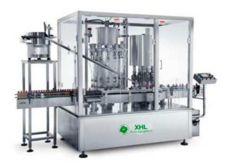
The washing, filling and turning integrated machine is mainly used for washing (water washing or air washing), filling, cap turning (capping) and sealing of oral liquids, syrup, medicinal wine, health products and tincture for external use in such industries as medicine, food, health products, etc.
