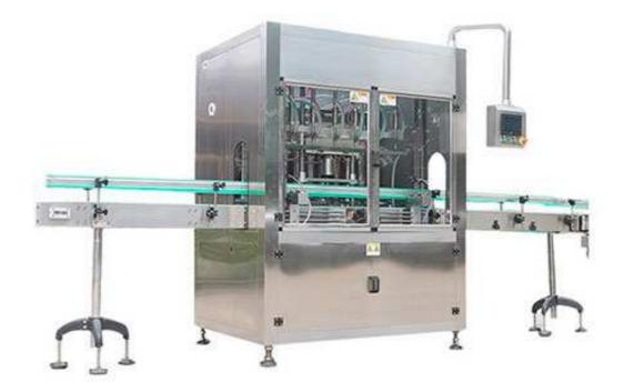
Piston Filling Machine Is Usually Used For Oil And Other Liquid With Higher Viscosity Like Salad Dressings, Peanut Butter, Potato Salad. With Glass Bottle, The Cap Could Be Crown Cap, Screw ROPP Cap, Pull-Ring Cap, Or Twist Off Cap.
