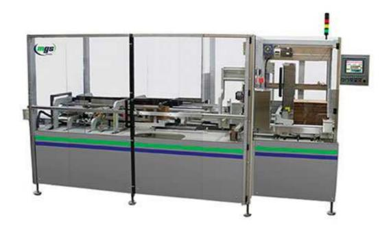
The MGS Machine Model MatriX<sup>™</sup> is a case packer capable of speeds up to 15 CPM.
