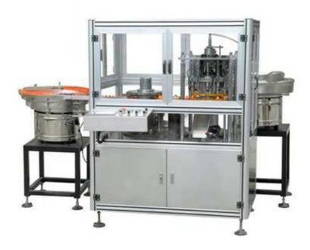
This cap assembly machine can assemble all kinds of plastic bottle caps, and can smoothly assemble the inner and outer parts of ejector caps, implosion caps, caps with explosion-proof rings and anti-counterfeit tooth caps.
