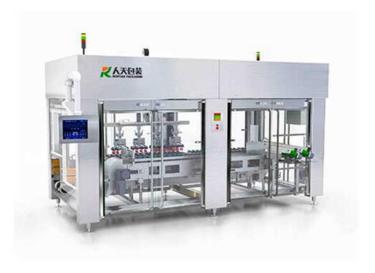
The machine is used to pack and arrange soft bags, strips, blocks, boxes and other materials. It adopts top-loading packing type and can rapidly achieve the changing of materials and mode of packing. Accuracy, high speed arrangement and packing can be achieved through material arrangement by race tracker, material picking and placing by rectangular coordinate robot, and carton supply and positioning device.
