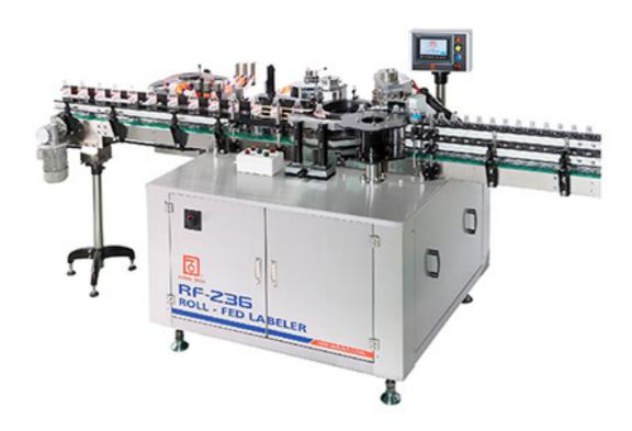
Suitable for 250cc~1500cc (bottle diameter 50mm~90mm) filled or un-filled round bottle shape labeling application as mineral water bottle, drink bottle, glass bottle, PET bottle, stable speed reaches to 200~300 BPM.
