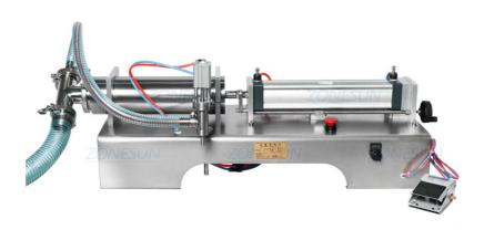
Compared with before pneumatic filling machine, this liquid filling machine is controlled by air pressure totally. The machine body may get heated due to the electricity. So this full pneumatic filling can ensure the machine body is cool during working. It is designed for filling flammable liquid like alcohol.
