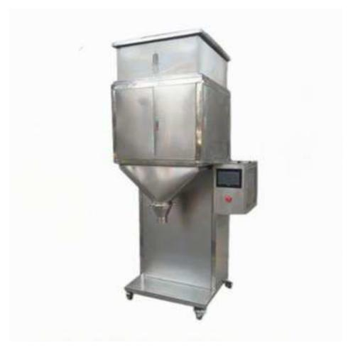
It is suitable for quantitative packaging of peanut, melon seeds, seeds, fertilizers, pesticides, grain and other granular, coarse powder materials. Combining self-flow cutting with vibration cutting, electronic weighing and metering is fast and accurate
