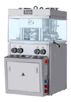
It is a new type double-sided multi-functional tablet press machine, which can press hard-forming raw material into big size tablets, such as milk tablets, effervescent tablet, calcium tablet, dishwashing tablet, salt tablet, ect.
