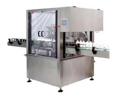
Gear pump filling equipment is exclusively designed to fill different types of liquid such as diesel oil, crude oil, lube oil, cacao butter, vegetable fats, animal food, acid, soap, and many more products. It is perfect filling machine applicable in wide range of industries which has requisites for filling liquid products.
