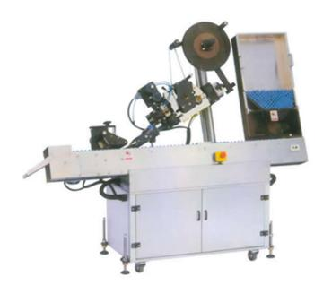
With bottle supplying equipment and roller chain conveyer belt, we can complete putting bottles, delivering bottles and sticking label at one time. Add stick rolling equipment, it can do wrap around stick, half wrap around stick. We also can attach printer. It suits for some object that is unable to stand or stand non-steady.
