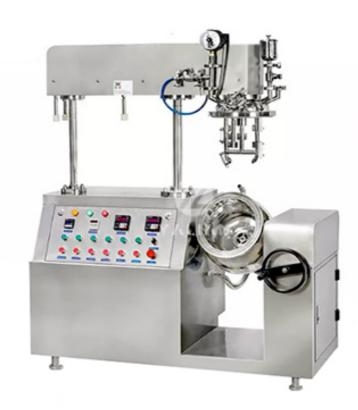
5/10L vacuum emulsifying machine is the necessary equipment for producing various ointments, ointments, cosmetics, cream and other emulsified products; the machine is simple in structure, easy to operate, novel in appearance and reliable in performance. It is the best choice for experiments and small batch production of customers such as pharmaceuticals, biology, cosmetics, chemicals, food, petroleum, etc.
