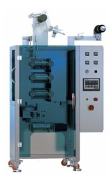
YS-186 is suitable for packaging of food, cosmetic powder, liquid, sauce and other items. It can automatically complete bag making, metering, blanking, sealing, slitting, counting, and can be configured to print batch numbers and other functions according to customer requirements. Use touch screen to operate PLC control, drive servo motor to control bag length, stable performance and easy adjustment.
