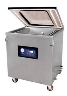
Vacuum packaging machine with trolley and double lateral sealing bars, made of stainless steel (AISI 304). Equipped with digital panel and volumetric electronic sensor for the steady control of vacuum. Volume increased chamber and convex lid for a max height of 250 mm. The vacuum pump of 40m3/h with three-phase 380 V motor ensures high productivity.
