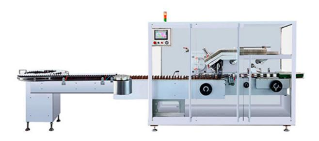
YL-130 Automatic Cartoning Machine is suitable for automatic feeding round bottle/square bottle into carton which bottle use in pharmaceutical, cosmetic, food, health product. On line bottle unscramble and feeding, leaflet fold (1-4 folds) and feeding, leaflet detecting, canton opening and forming, products and leaflet pushing into carton, printing batch number, sealing carton with tuck-in or hot melt glue device. Automatically reject lacking of leaflet or product and finished product out.
