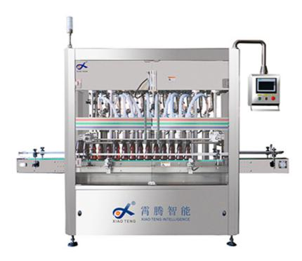
The machine adopt servo motor driven, containers will be sent to the position, then the filling heads will dive into the container, filling volume and filling time can be set in orderly. When it filled up to the standard, servo motor go up, container will be sent out, one working cycle is finished.
