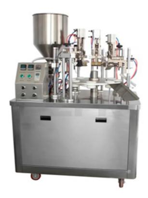
The NF-30 aluminum tube potting machine is mainly used for the primary transmission principle. The indexing mechanism is used to drive the rotary table equipped with the clamp for intermittent movement, and the automatic filling and the two sides of the tail, the three-side folding tail and the saddle-shaped folding and sealing work are completed. The shape and size of the seal can be easily and accurately adjusted according to the needs of the user.
