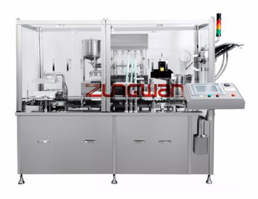
Automatic machine firstly developed in china by zhonghuan, Features include automatic syringe nest-tubin-feeding, automatic vacuum filling, automatic vacuum plugging and automatic operation with monitoring all the way. Beside normal liquid, also suitable for filling transparent thick liquid like ester acid.
