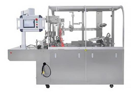
TMP-400S mechanical high-speed automatic transparent film three-dimensional packaging machine can automatically feed, wrap, fold, side seal, end seal, up and down shaping, count and automatically paste anti-counterfeiting easy-pull lines and surfaces for single-box and multi-box collections. The functions of ironing and spot ironing make the operation, adjustment, mold replacement and maintenance of the whole machine more convenient and quick.
