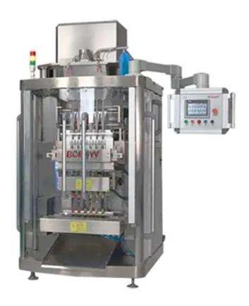
BVS6-680 is specially designed for stick bags, and can be made into larger stick bags. 2-12 lane can be selected according to customer needs. The edge sealing shape and pattern of the bag can also be changed. It can package powders, granules, liquids and other materials, and it occupies a small area and is easy and quick to operate.
