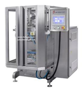
The HSD-510 Continuous High-speed Vertical Packaging Machine is a continuous motion vertical form fill seal packing machine. It utilizes a draw bar pulling mechanism which includes a hydraulic draw bar which moves vertically up and down, and pull the film with the end seal jaws. Speed up to 180 bags per minute.
