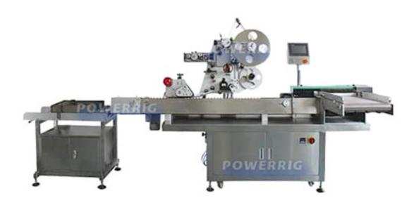
A high-speed servo horizontal labeling machine is an advanced industrial machine used for labeling products or packages horizontally at a high speed. It incorporates servo motor technology, which provides precise control and synchronization for efficient labeling operations. This type of machine is commonly used in industries such as food and beverage, pharmaceuticals, cosmetics, and logistics.
