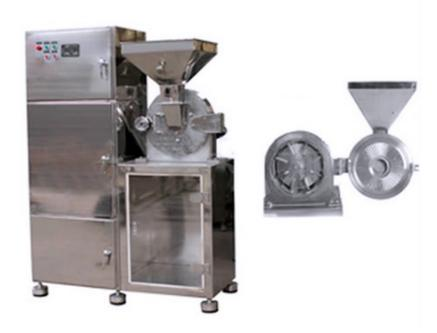
SF universal pulverizing machine uses high-speed relative motion between movable and fixed teeth discs. Raw materials will be impacted by teeth and frication. Finally they are crushed. Universal pulverizer is widely used for pharmaceutical industry, chemical industry, pesticide industry, foodstuff industry, grain industry, and so on.
