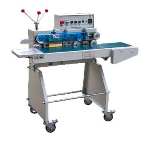
The SA-113 Continuous-Type Sealing Machine is designed to seal bags. After putting food into bags, align the open end with the sealing conveyor to let the conveyor convey and seal the bags. The sealing machine is equipped with a printing device for printing expiry date right after sealing.
