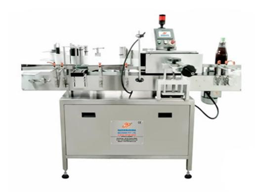
The Automatic Sticker Labelling Machine consists of a main structure, product transmission belt with an adjustable guide, separator unit, label dispenser unit, label wrapping unit, electrical panel, PLC & HMI, AC drives & a batch printing unit (OPTIONAL). The complete operation is PLC-based.
