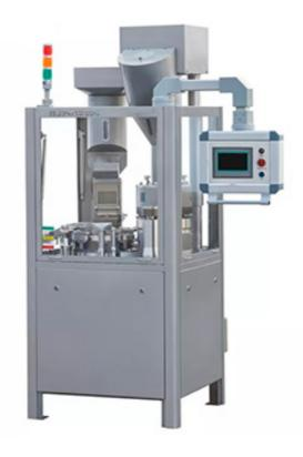
The machine is an intermittent motion and hole plate type filling fully automatic capsule filling equipment.
