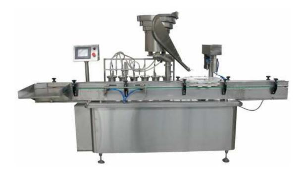
This machine is the main filling equipment of the oral liquid production line, which is mainly applied in the filling, covering and sealing of the 30 - 500 ml bottles. This machine combines filling and sealing, advanced design, compact structure, the Replacement of the bottle is very convenient.
