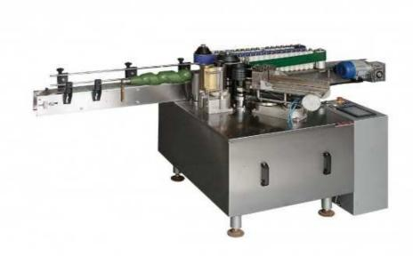
Labeling machines are applied to various operations such as sticking a label on plane, post surface, single side or multi-sides of a package, sticking labels covering part or all of the surface of a cylinder, or sticking on sunken locations and at edges or corners.
