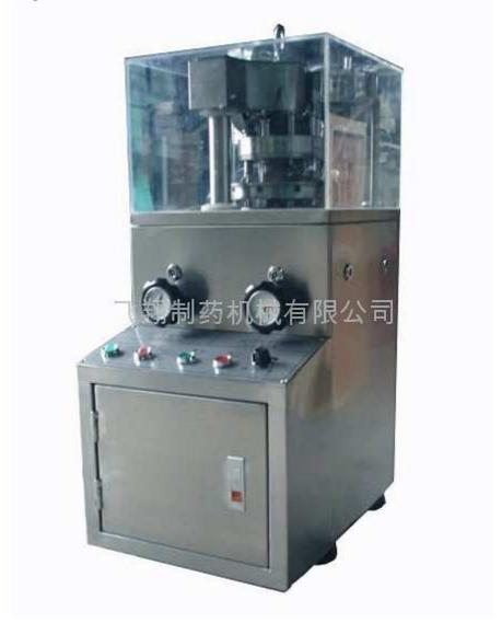
This machine is a single press type, continuous automatic tablet press for pressing granular materials into various tablets, such as round or irregular tablets.
