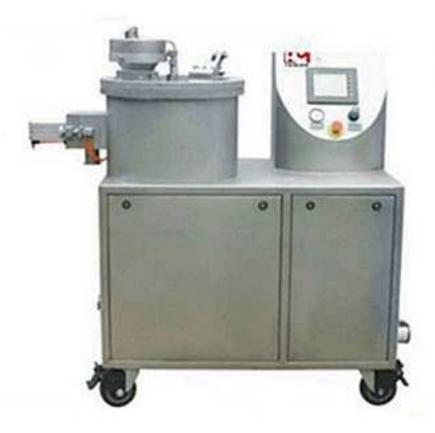
**Usage:** spheroidize compact cylindrical granules to get final pellet
