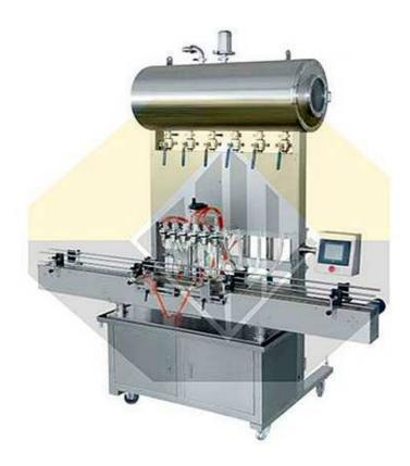
VFC-6 Automatic 6 Heads (Piston) Cream Filling Machine is widely used for daily chemicals, foodstuffs, pharmaceutics and oil. It can filling various kinds of cream, the filling volumes range is 25-5000ml, the max filling speed can reach 40 bottles/min.
