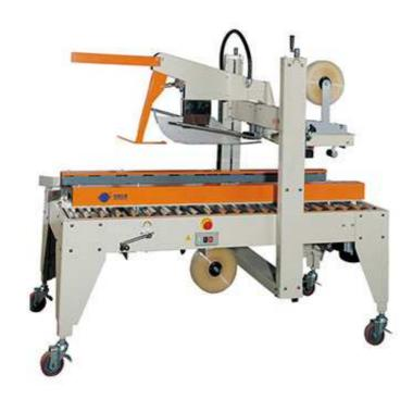
Fit for sealing uniform size carton in mass production line. Automatic flaps folding and, top and bottom sealing Side belts driven, suitable for heavy duty operation.
