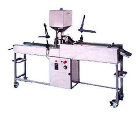
This inspection machine is designed and used for inspecting capsule or tablet which is spotty, broken or not standard by vision through mechanically rotating the capsule over 360 degrees or turning the tablet from one surface to the other surface. Inspection can be easily determined.
