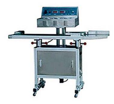
This series Continuous Induction Sealer Machine utilizes electromagnetic induction principle to produce instant high heat to melt aluminum foil that then adheres to the bunghole, reaching the aim of wet-proof, leakage-proof, mildew-proof and extending preservation time. Now it is widely used as sealing package machine in industries such as pharmaceuticals, pesticides, pesticides, lubricant and cosmetics etc.
