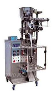
The MK-211 is a fully pneumatic vertical form fill and seal (VFFS) packaging machine designed to package granular and free flowing powdered products. This Fully automatic vertical packaging machine uses volumetric cup dosing system to produce center sealed, 3 side sealed and 4 side sealed pouches / bags.
