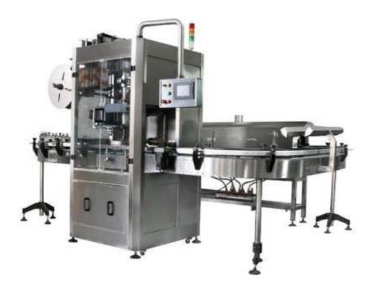
Within a certain diameter range, this machine can be used for many types of bottles: round, square, oval, conical or other irregular shapes.
