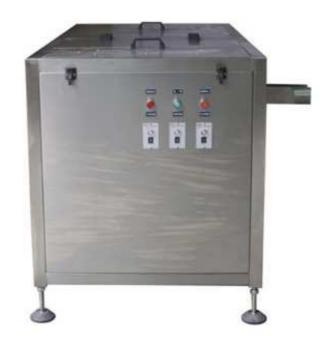
DLP-200B large bottle arranging machine for round bottle of beverage industry, large capacity high-speed rationale bottle, to more than 1L bottle of bottle handling speed up to 120 bottles / minute above.
