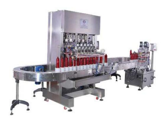
The filling and capping machine is one kind of automatic production equipment. This filling machine is suitable for different viscosity liquid. It adopts pneumatic piston type filling. Volumetric measurement and Proximity switch control the piston to filling. It can ensure the filling precision. It widely apply to fill the food, pharmaceutical, daily chemical, pesticide, cosmetic and other liquid or viscosity cream.
