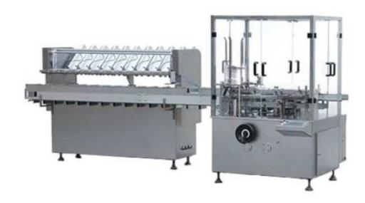
This machine is suitable for scotch, punch, soft al/al strips, wound pester, ointment plaster, facial mask, coffee bags into carton automatically. On line product feeding and detecting, carton opening and forming, products and leaflet push into carton, printing batch number, sealing carton with tuck-in or hot melt glue device. Automatically reject lacking of leaflet or product and finished product out.
