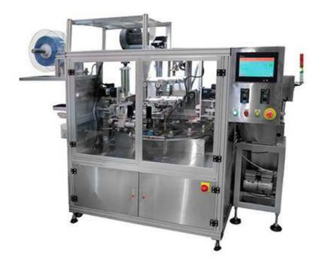
Adhesive Tape Shrink Sleeve Applicator, LR-100 is specially designed by inserting shrink band, placing paper label & shrinking full packaging process for tape. Modularized main machine & mechanism are easy adjustment & quick change. Its cutter is designed particularly for easy replacing to save time. Al control system can be installed to help smart production.
