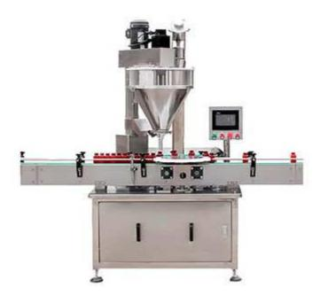
Automatic auger filler machine of model VTOPS-PSH-02 is a rotary type automatic auger filler. It is a new style automatic powder bottle auger filler machine which developed by Zhengzhou Vtops Machinery Co., Ltd. The single head automatic auger filler using rotary indexing Star-Wheel.
